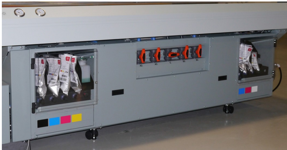
19. Ink Bays and Vacuum Zone Control Handles
